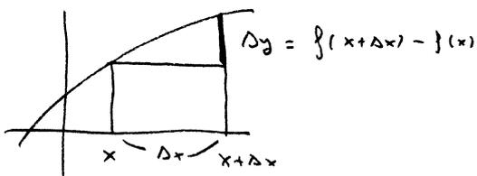
$$f'(x) = \lim_{\Delta x \rightarrow 0} \frac{f(x + \Delta x) - f(x)}{\Delta x} = \lim_{\Delta x \rightarrow 0} \frac{\Delta y}{\Delta x}$$
