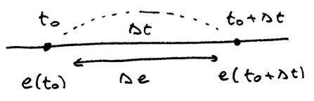
$$v_{t_0} = \lim_{\Delta t \rightarrow 0} \frac{\Delta e}{\Delta t} = e'(t_0)$$
